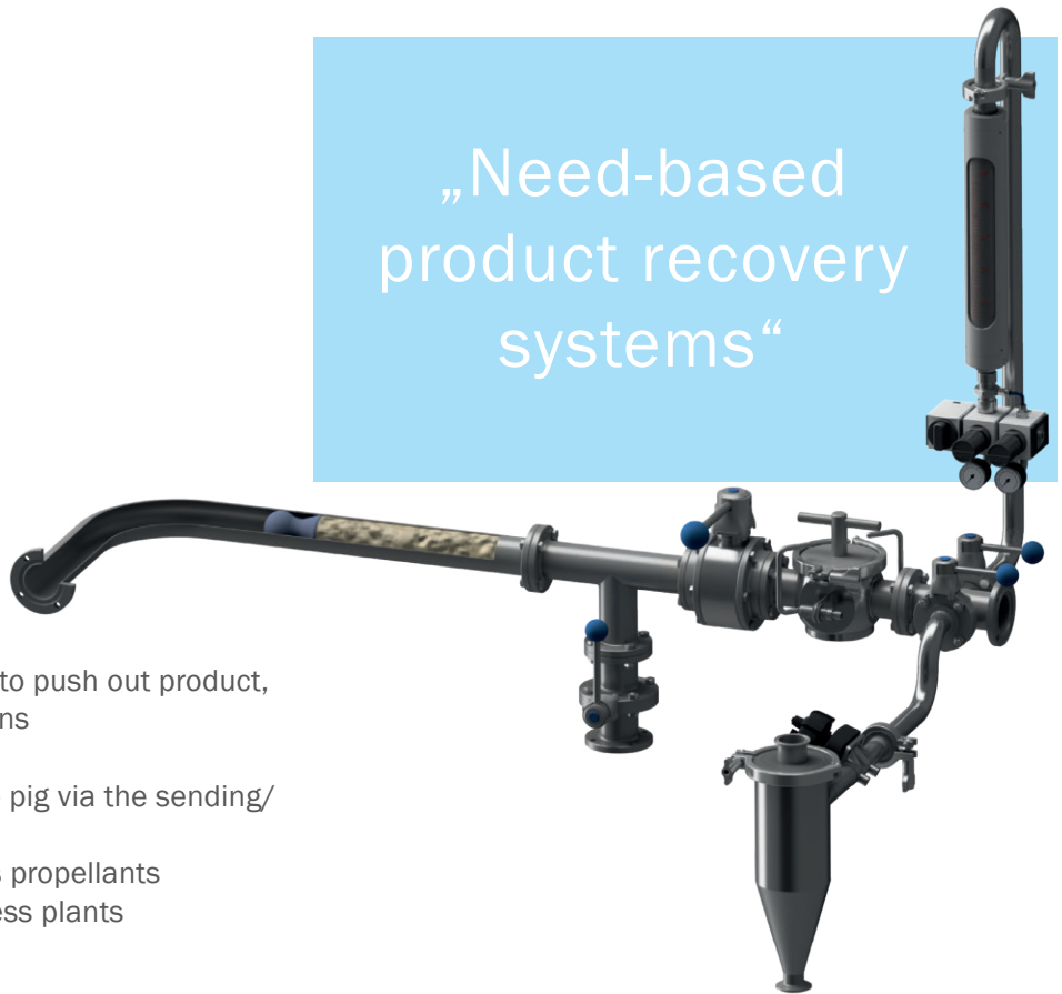
Manually operated product recovery system: illustration of a sending/receiving station with piggable T-piece and ball valve as well as product valve, propellant supply, and relief via cyclone
